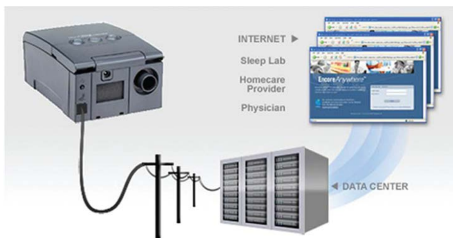
Figure 35. Equipment for continuous positive airway pressure telemonitoring based on modem technology (Encore Anywhere™; Philips Respironics, Murrysville, PA, USA) ( Sparrow et al., 2010 ).
